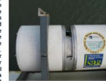
Figure 1: Image of the jammed shutter on the Pride of Bilbao as found on 15.06.2004. After the recovery a were carried brations in the facilities at the aphic Centre if the instrument behaviour under deployment temperature ach was done for the ambient temperatures of 10, 15 and
