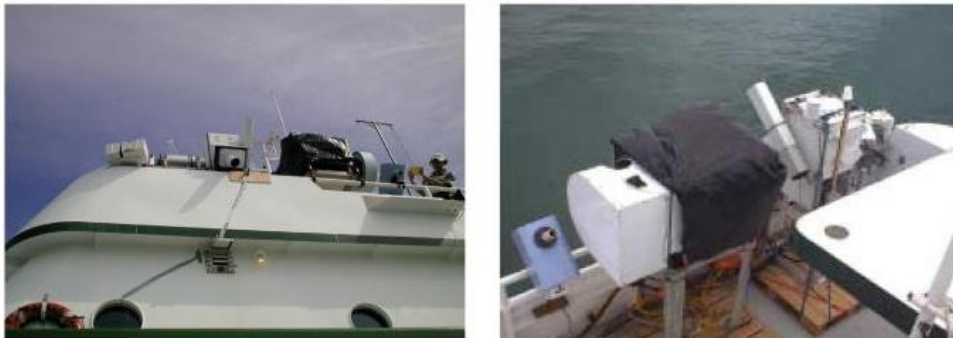
Figure 4. Left – the infrared radiometers mounted on the upper deck. From the left these are SISTeR, ISAR, CIRIMS, M-AERI, DAR011, and the hand-held TASCO. Right – the view from above. The JPL radiometer was mounted on the fore-deck, viewed the sea between the two hulls of the Walton Smith , and is not visible in these photographs.
