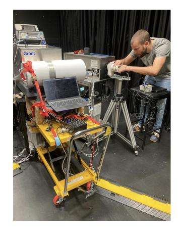
Radiometer Measurement against reference BB source at NPL during June- 2022 Radiometer Intercomparsons. Ref: FRM4SST-CRICR-NPL-002\_ISSUE-1
